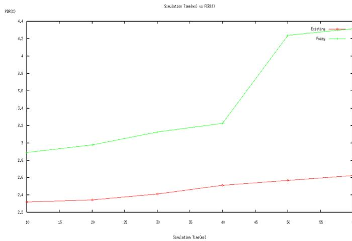
**Figure 5: Comparison of PDR between SCADA and Fuzzy Based Systems**
