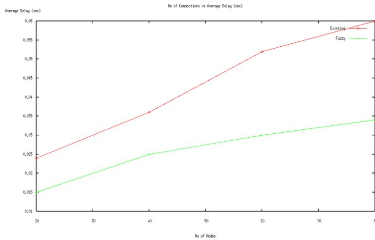
**Figure 4: Comparison of Delay Time between SCADA and Fuzzy Based Systems**
